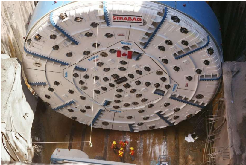
The 14.4-meter diameter TBM 'Big Becky' utilized at Niagara.. Source: Bloomberg / Bloomberg via Getty Images
