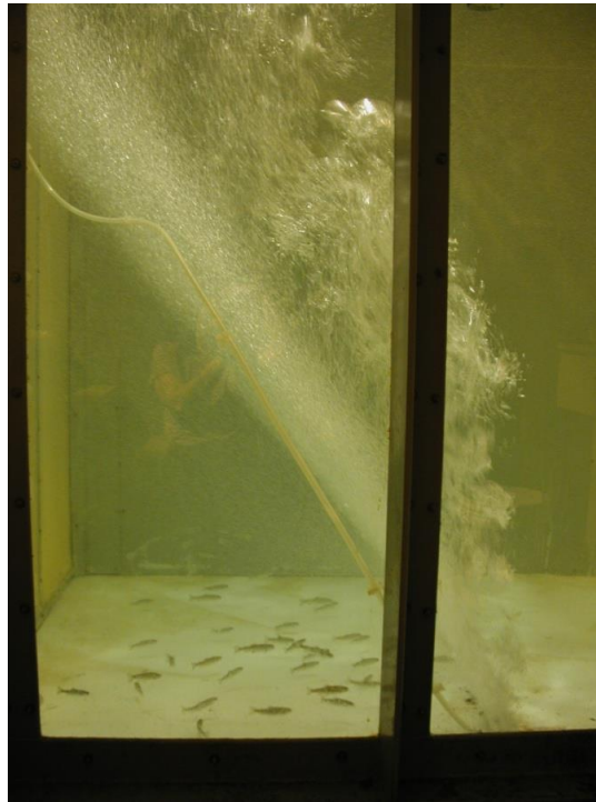
Figure 4-2 Air Bubble Curtain (Courtesy of Alden)
