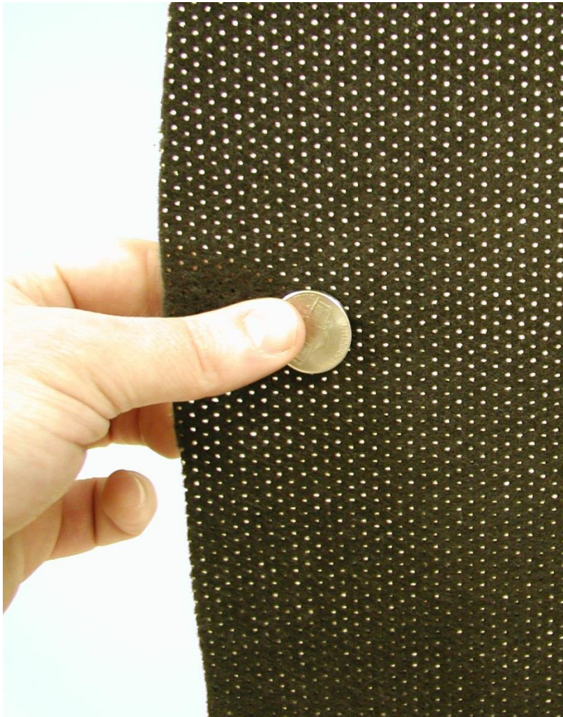
Figure 4-20 Close-up of Perforated AFB Material (Courtesy of Alden)
