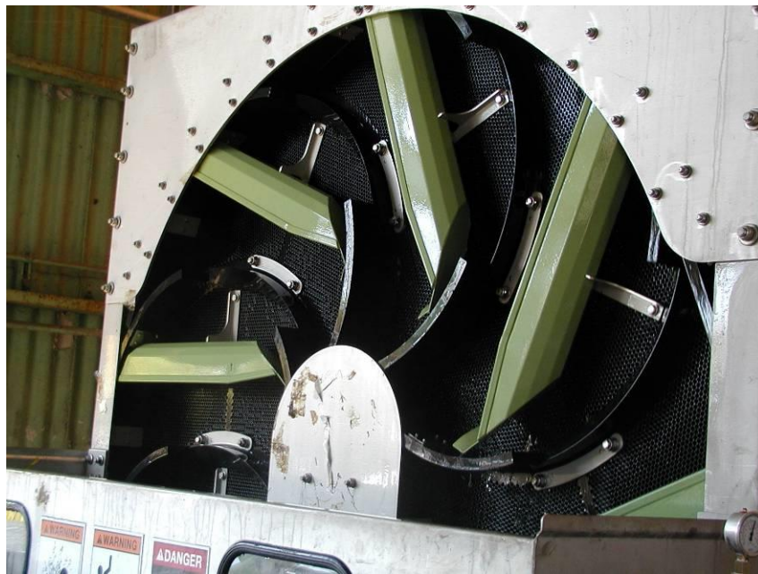
Figure 4-8 Bilfinger Multi-Disc Screen with Fish Lifting Buckets (Courtesy of Bilfinger)
