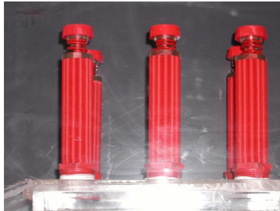
Figure 4-18 Filtrex Filter Elements (Courtesy of Alden)
