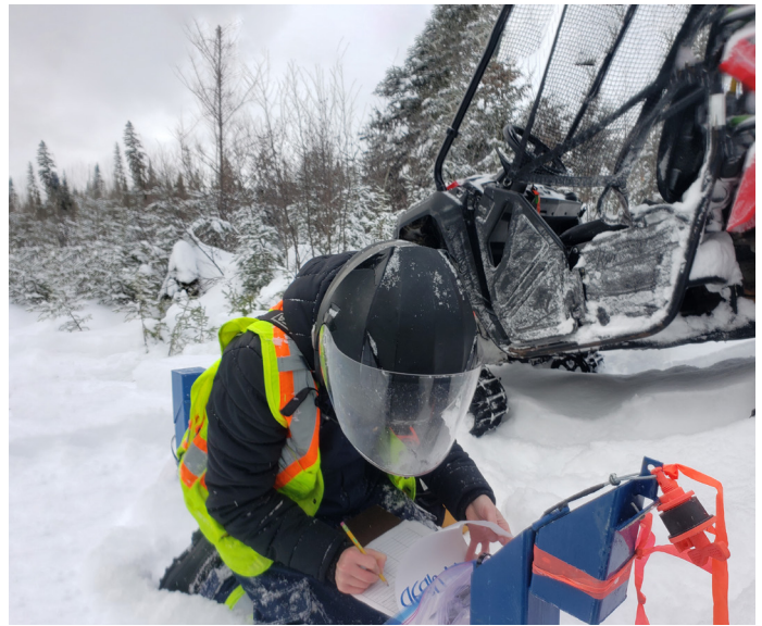
Groundwater level monitoring during a pump test.
