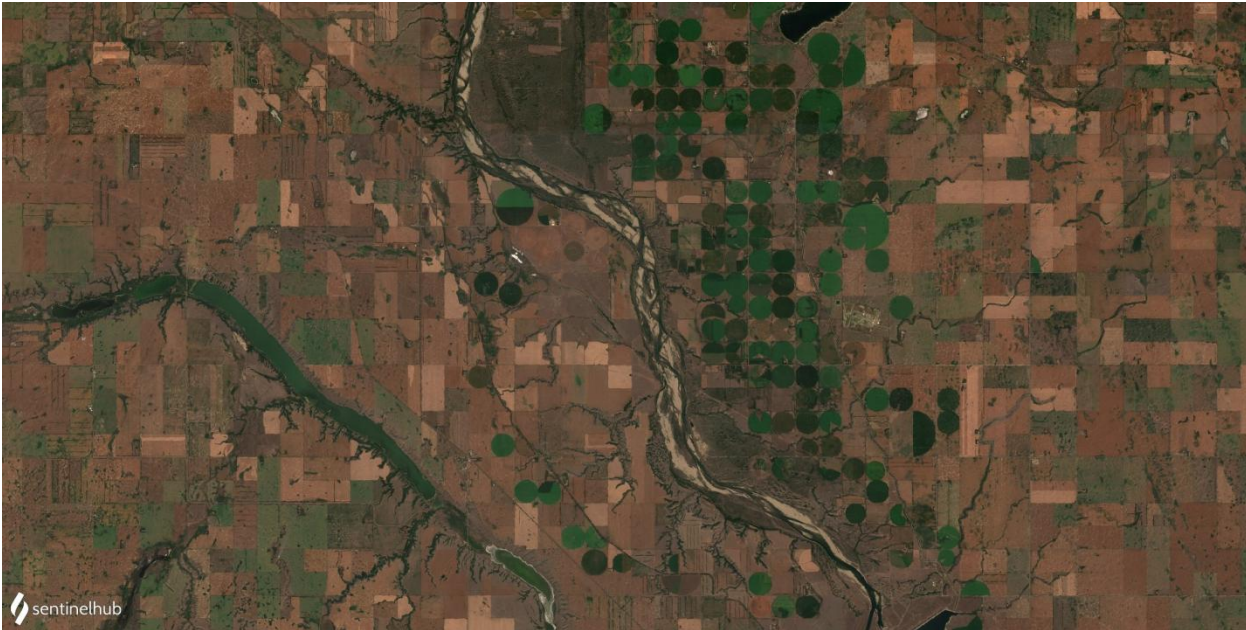
245 Figure 5. Sand and silt build up in the South Saskatchewan River immediately downstream of the Gardiner Dam on Lake Diefenbaker and adjacent to the regional irrigation districts
