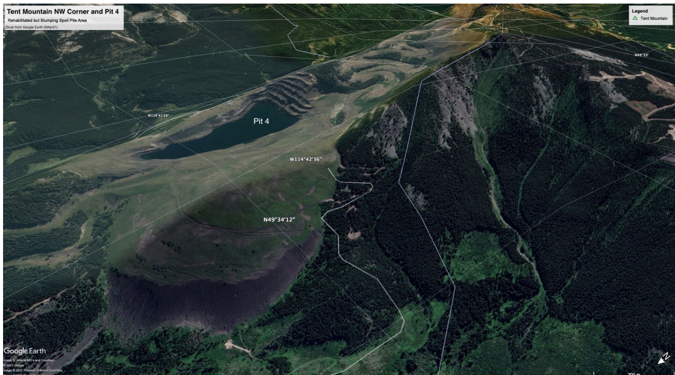
Figure 4: Tent Mountain NW section and Pit 4. Waste Rock spoil shows slumping and erosion.
