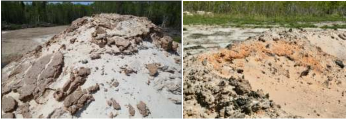
Figure 6. Concretions potentially containing sulphide in pyrite and marcasite in sand piles extracted near Vivian, Manitoba in the spring of 2020.
