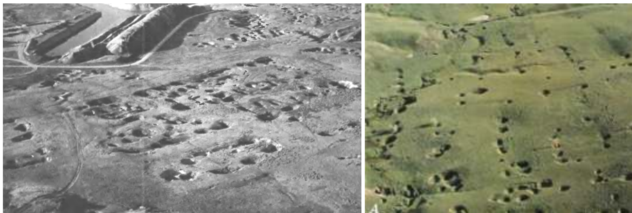
Figure 5. Subsidence and sinkholes at Sheridan, Wyoming from an abandoned underground coal mine 27
