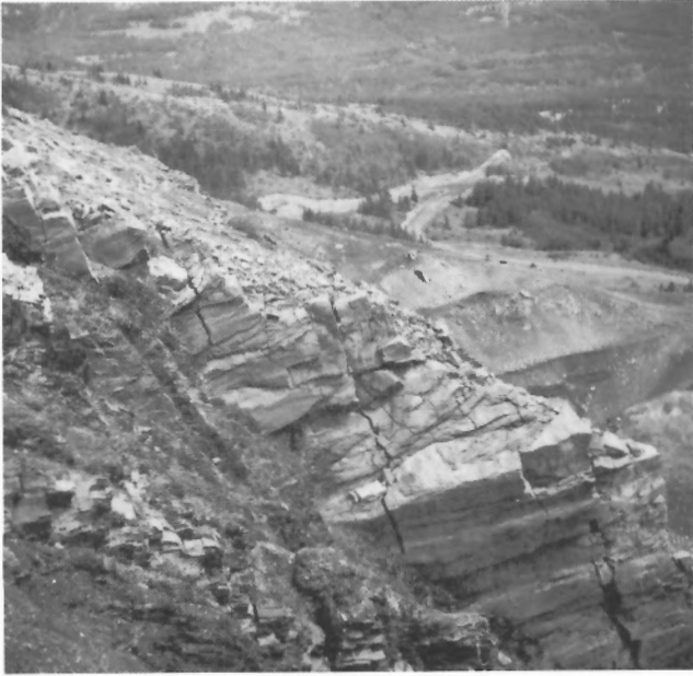
Figure 11. Family of extension faults in sandstone on top of No. 2 Seam on the east flank of the "Pod", No. 2 Pit, Grassy Mountain. GSC photo. 117445.
