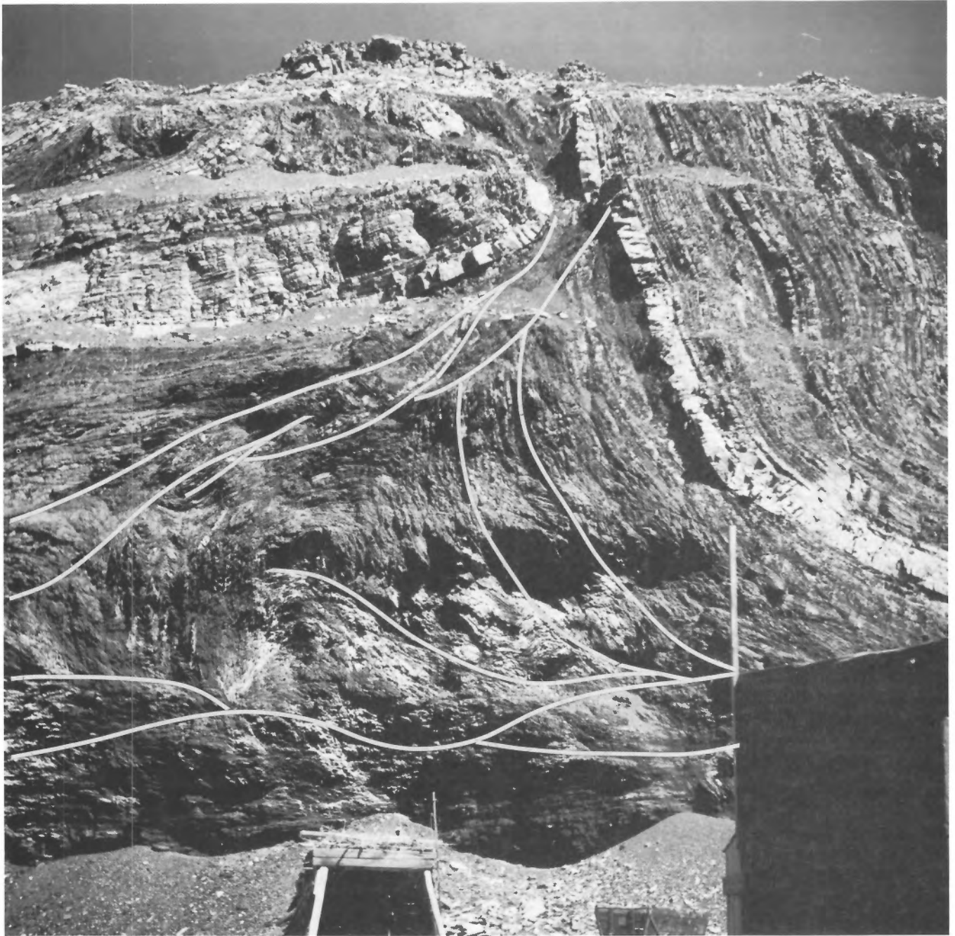
Figure 26. Structural thickening of No. 2 Seam coal in the hinge of Grassy Mountain Anticline, No. 2 Pit, Grassy Mountain. White lines identify some of the contraction faults along which slices of highly sheared coal have been displaced, from both sides, toward the hinge of the fold. GSC photo. 117435.
